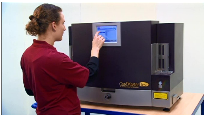
Figure 10 – The operator controls the system via a touch screen
